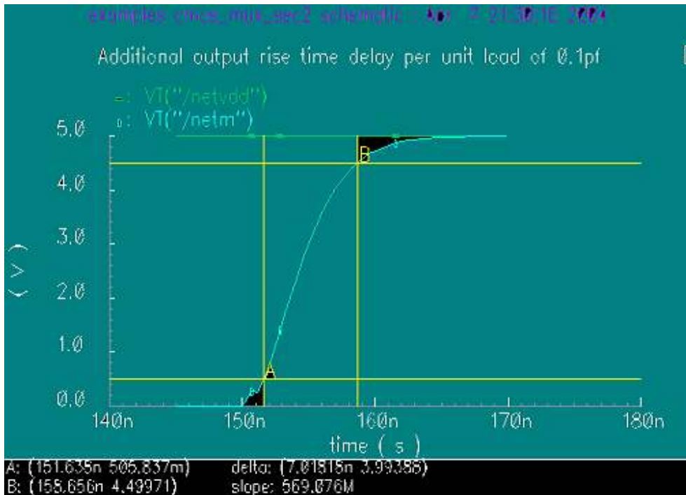
2.7 Additional output rise time delay per unit load of 0.1pf (7.0ns)
