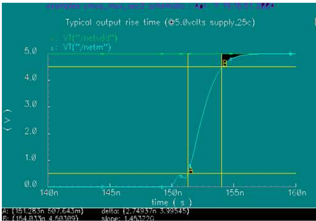
2.2 Typical output rise time (2.75ns)
